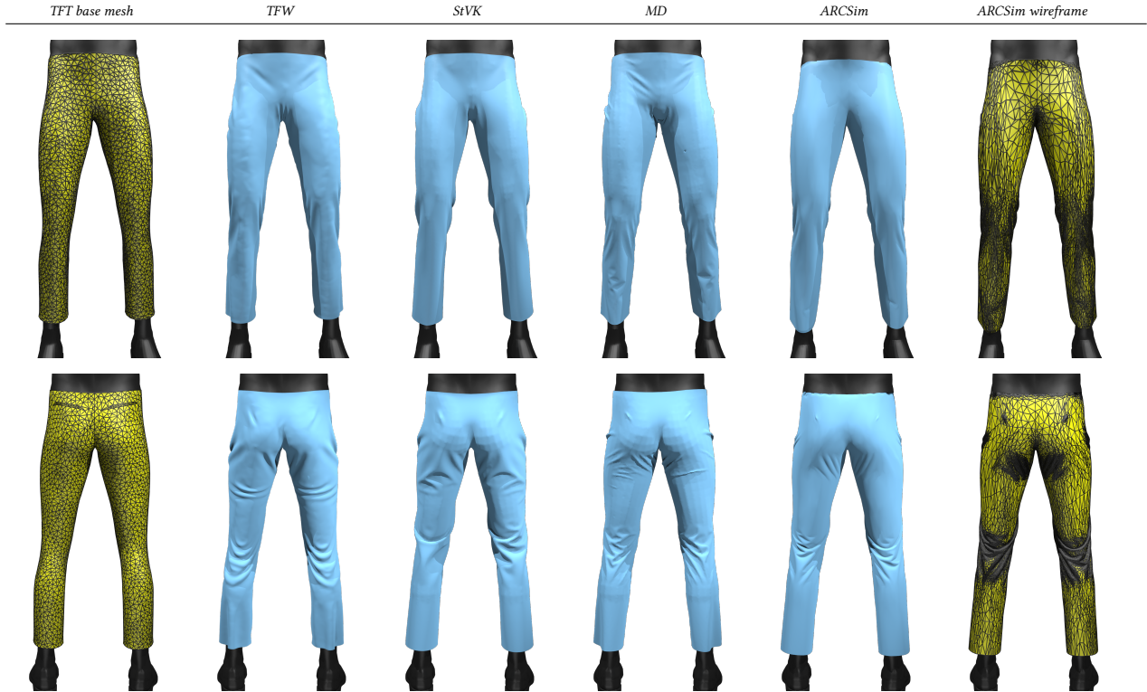
Fig. 16. A mannequin wearing simulated pants. The first row shows the front view of the pants after simulation and the second row shows the back view of the same pants. From left to right: a 4k-vertex base mesh, simulated using TFT ; the simulated wrinkled shell using TFW on that base mesh; the result from StVK on a Delaunay mesh with 60k vertices; the result from MD on a 60k-vertex mesh; the result from ARCSim , with adaptive remeshing enabled; a wireframe rendering of that same ARCSim result (the mesh has 15k vertices). For StVK and MD , we tuned mesh resolution to be about as coarse as possible without causing significant degradation in the wrinkle pattern.
