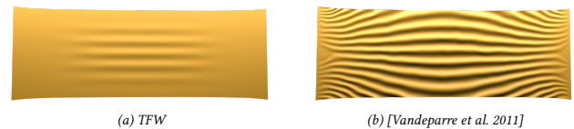
Fig. 8. Comparison of (a) our method and (b) wrinkles generated using the scaling law of Vandeparre et al. [2011] for the model problem of a highly stretched sheet [Wang et al. 2018]. In examples where the wrinkles are not caused by wrinkles propagating inward from a clamped boundary, the analysis of Vandeparre et al. does not apply.
