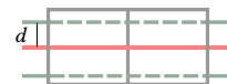
Fig. 4. The d -iso-surface (green lines) of the input mesh (red line) cannot be captured if the voxel size is larger than 2d .
