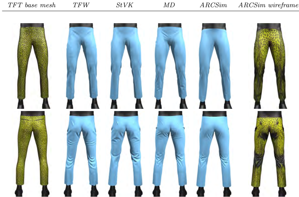
Figure 2.15: A mannequin wearing simulated pants. The first row shows the front view of the pants after simulation and the second row shows the back view of the same pants. From left to right: a 4k-vertex base mesh, simulated using TFT ; the simulated wrinkled shell using TFW on that base mesh; the result from StVK on a Delaunay mesh with 60k vertices; the result from MD on a 60k-vertex mesh; the result from ARCSim , with adaptive remeshing enabled; a wireframe rendering of that same ARCSim result (the mesh has 15k vertices). For StVK and MD , we tuned mesh resolution to be about as coarse as possible without causing significant degradation in the wrinkle pattern.
