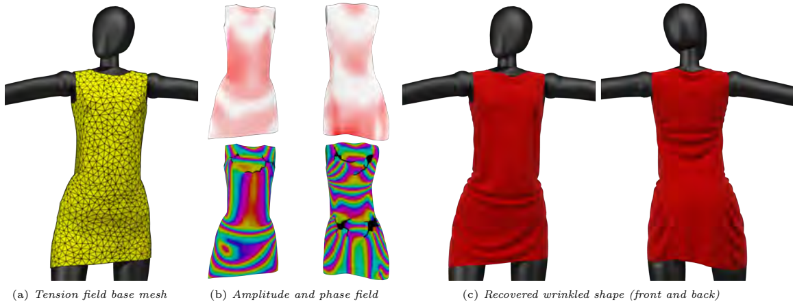
Figure 2.1: Overview of our pipeline for predicting the wrinkled equilibrium shape of a thin shell (in this case, a cloth dress draped on a mannequin). We approximate the coarse shape of the draped cloth using tension field theory (a), in which material forces do not resist compression. We then augment this base mesh , which can be very coarse (around one thousand vertices), with wrinkles. We formulate the elastic energy of the shell in terms of an amplitude (b, top ) and phase field (b, bottom ) over the base mesh, which together characterize the geometry of the wrinkles, and solve for these fields globally over the mesh. Our method recovers complex wrinkle patterns with nontrivial geometry and topology (c), including wrinkles with wavelength much smaller than the resolution of the base mesh.
