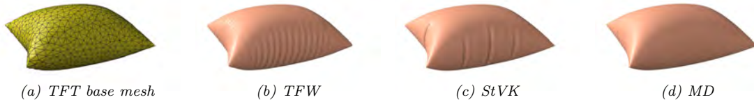
Figure 2.12: The simulated result of inflated teabags: (a) the TFT base mesh with 936 vertices; (b) shape recovered using TFW ; (c) StVK simulation on a 30k-vertex mesh, and (d) Marvelous Designer simulation with 30k vertices. Among all these results, StVK achieves the most natural shape (sharp creases + small wrinkles). TFW will need a much higher resolution to capture these sharp creases in the TFT base mesh.
