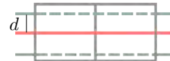
Figure 4.4: The d -iso-surface (green lines) of the input mesh (red line) cannot be captured if the voxel size is larger than 2d .
